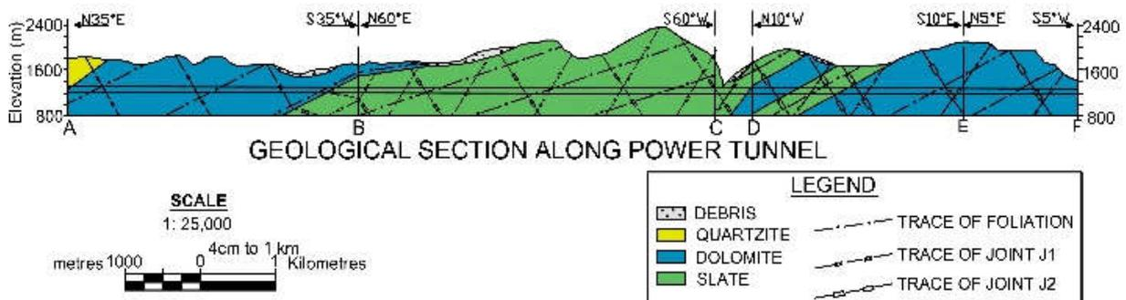
Fig. 3. Geological section along Power Tunnel
