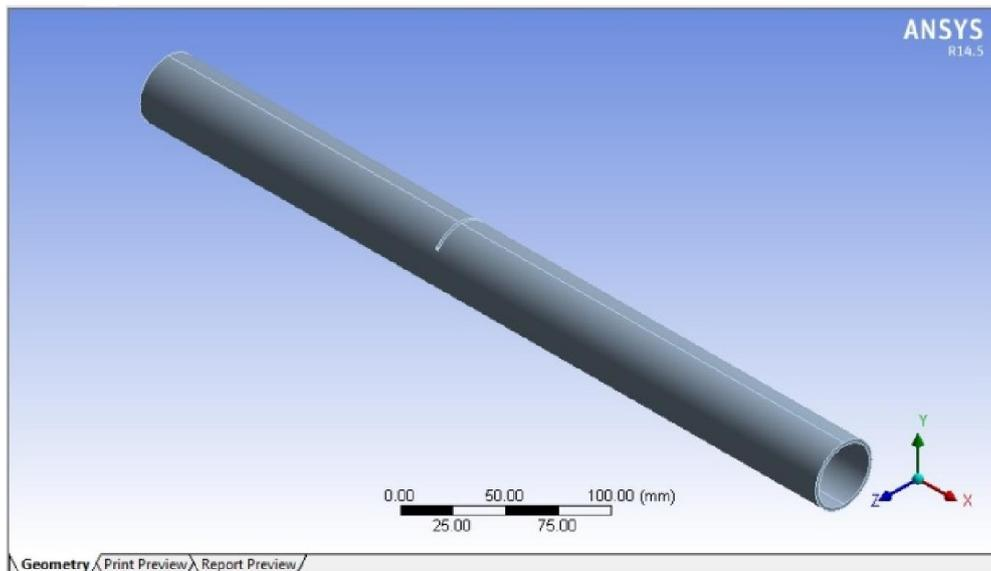
Figure 3. Cracked beam 8mm depth at 200mm from the fixed end
