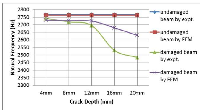
Figure 11. Effect of crack depth on the natural frequency of the second mode shape of a damaged cantilever beam at 100 mm from the fixed end
