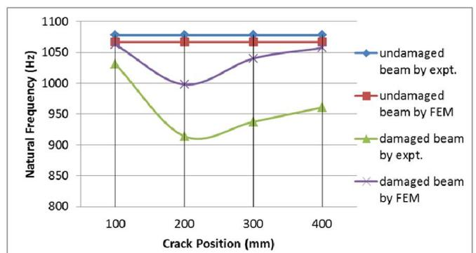
**Figure 15. Effect of crack position on the natural frequency of the first mode shape of damaged cantilever beam with 8 mm crack depth from the fixed end**
