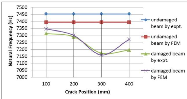
Figure 18. Effect of crack position on the natural frequency of the fourth mode shape of damaged cantilever beam with 8 mm crack depth from the fixed end
