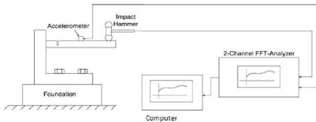
Figure 2. Experimental setup
