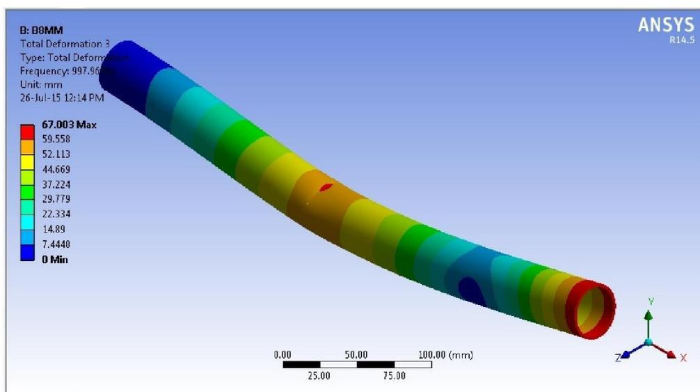
Figure 5. First mode shape of cracked beam
