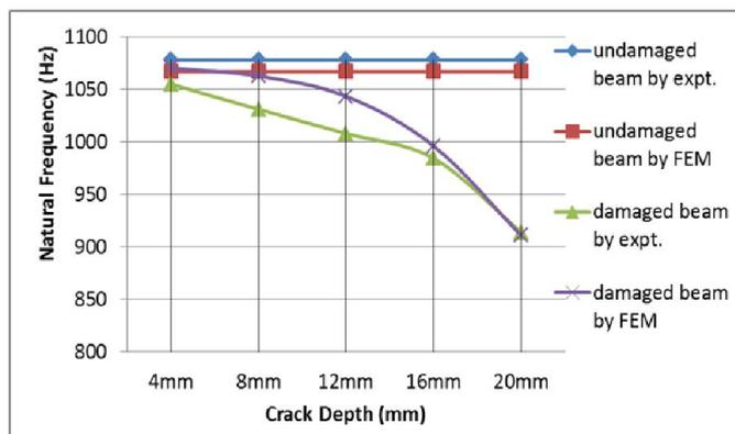
Figure 10. Effect of crack depth on the natural frequency of the first mode shape of a damaged cantilever beam at 100 mm from the fixed end
