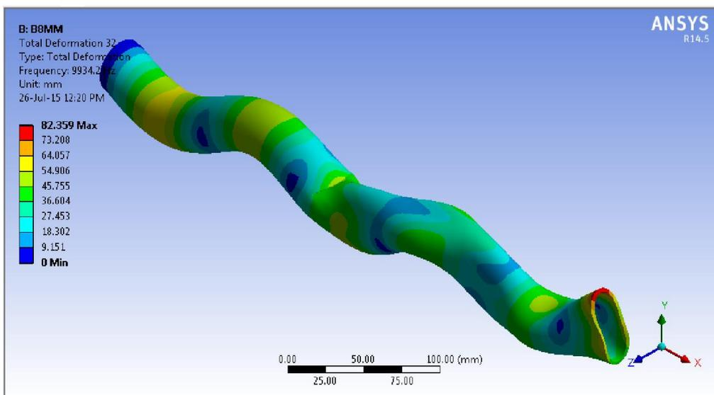
Figure 9. Fifth mode shape of cracked beam
