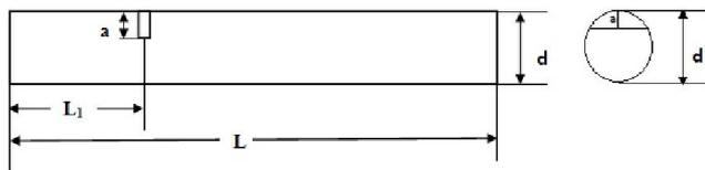
Figure 1. Geometry of beam with single crack
