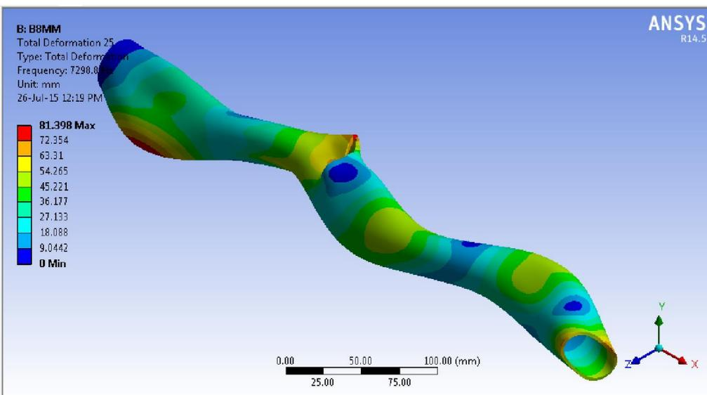
Figure 8. Fourth mode shape of cracked beam
