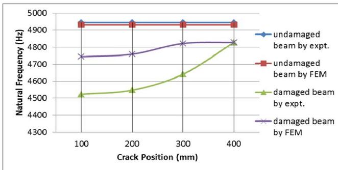
Figure 17. Effect of crack position on the natural frequency of the third mode shape of damaged cantilever beam with 8 mm crack depth from the fixed end
