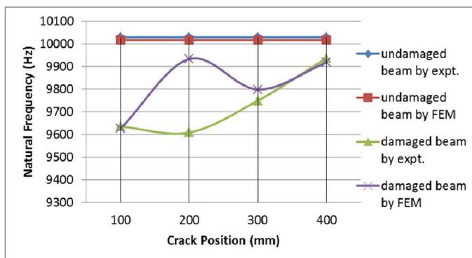
Figure 19. Effect of crack position on the natural frequency of the fifth mode shape of damaged cantilever beam with 8 mm crack depth from the fixed end
