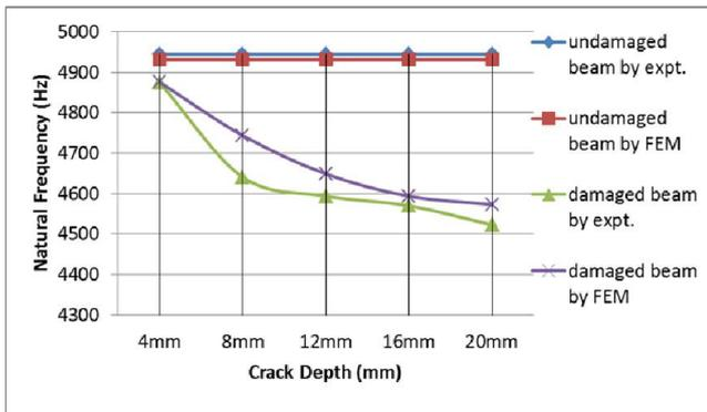
**Figure 12. Effect of crack depth on the natural frequency of the third mode shape of a damaged cantilever beam at 100 mm from the fixed end**
