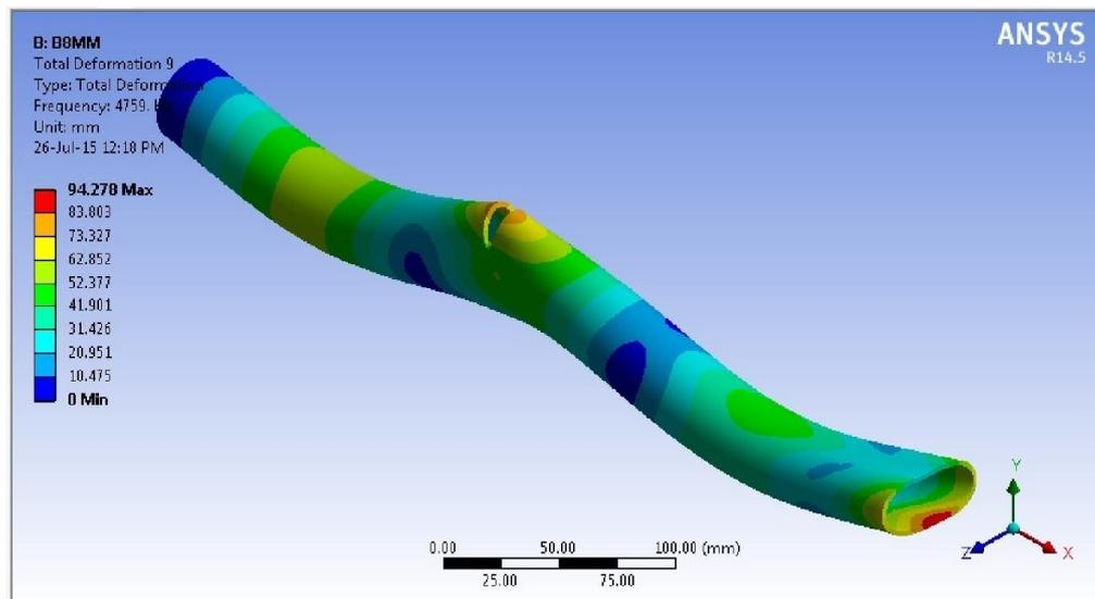
Figure 7. Third mode shape of cracked beam
