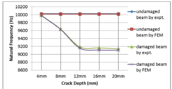
**Figure 14. Effect of crack depth on the natural frequency of the fifth mode shape of a damaged cantilever beam at 100 mm from the fixed end**
