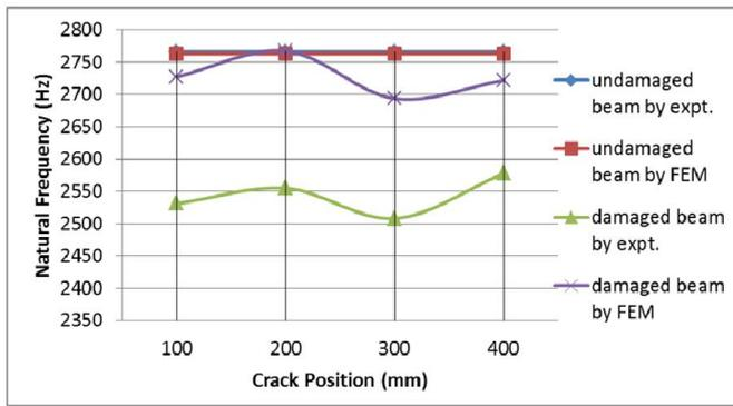
Figure 16. Effect of crack position on the natural frequency of the second mode shape of damaged cantilever beam with 8 mm crack depth from the fixed end
