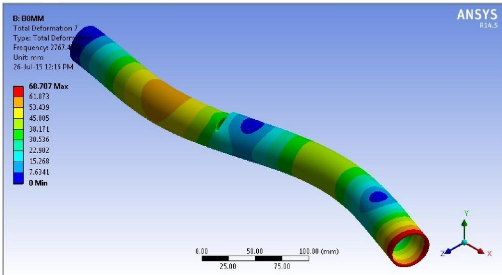
Figure 6. Second mode shape of cracked beam
