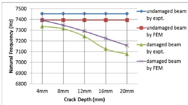
**Figure 13. Effect of crack depth on the natural frequency of the fourth mode shape of a damaged cantilever beam at 100 mm from the fixed end**
