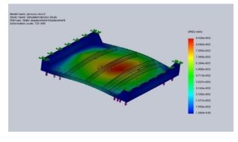
Fig. 9. Deformation of base with 4 ribs
