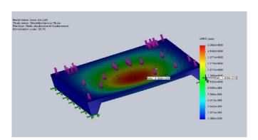
Fig. 3. Static deformation of base
