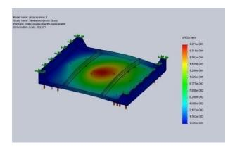
Fig. 7. Deformation of Base with 2 Ribs
