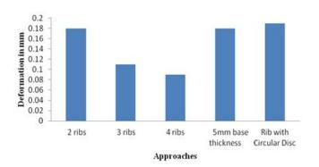
Fig. 11. Alternative Approaches vs deformation of canopy base
