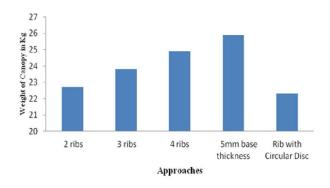
Fig. 12. Alternative Approaches vs Weight of canopy
