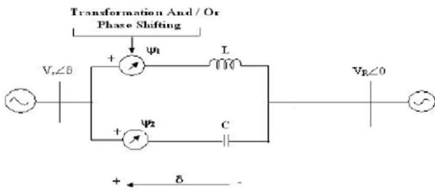
Figure 1. Operating Principle of IPC
