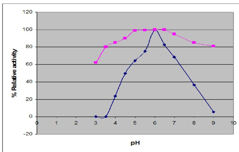
Fig. 7. Effect of pH on activity and stability of recombinant BGL1. For optimum pH, enzyme activity was measured in phosphate citrate buffer, pH 3.0 - 7.0 and pH range of 8.0-9.0 at 50 °C
