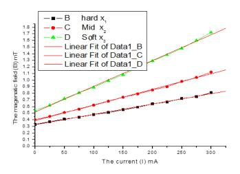
Figure 2. The relation between magnetic flux B and Current Ifor different size Iron Fillings
