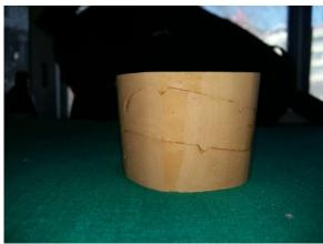
Fig. 8. Three piece mold fabricated
