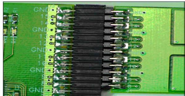
Fig. 17. Interfacing channels with 8-key touch board
