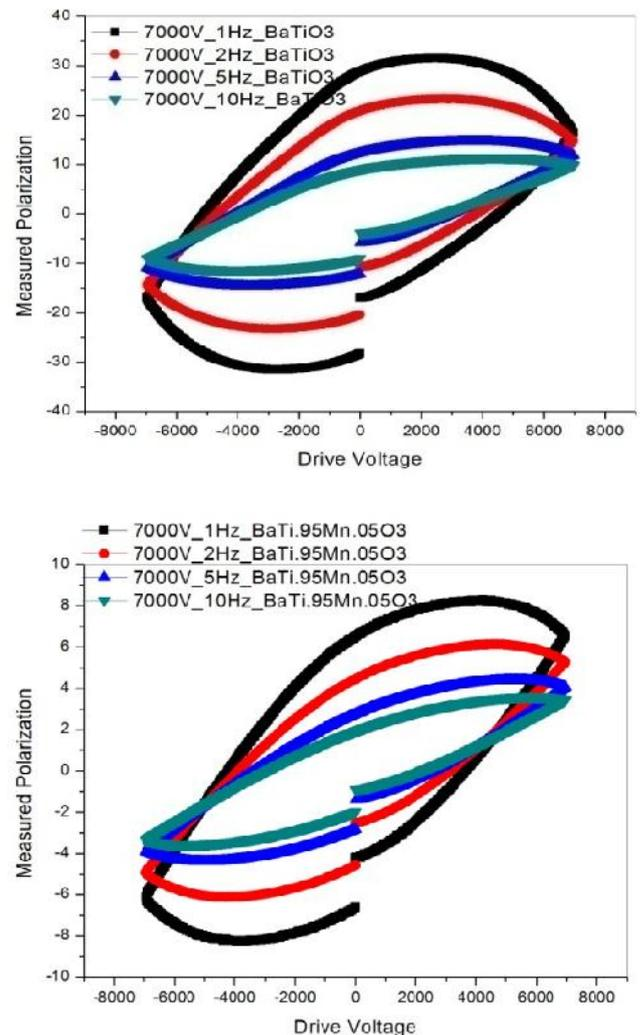
**Figure 5. The room temperature P-E loops of (a) BaTiO<sub>3</sub>, (b) BaTi<sub>0.95</sub>Mn<sub>0.05</sub>O<sub>3</sub> ceramic samples**
