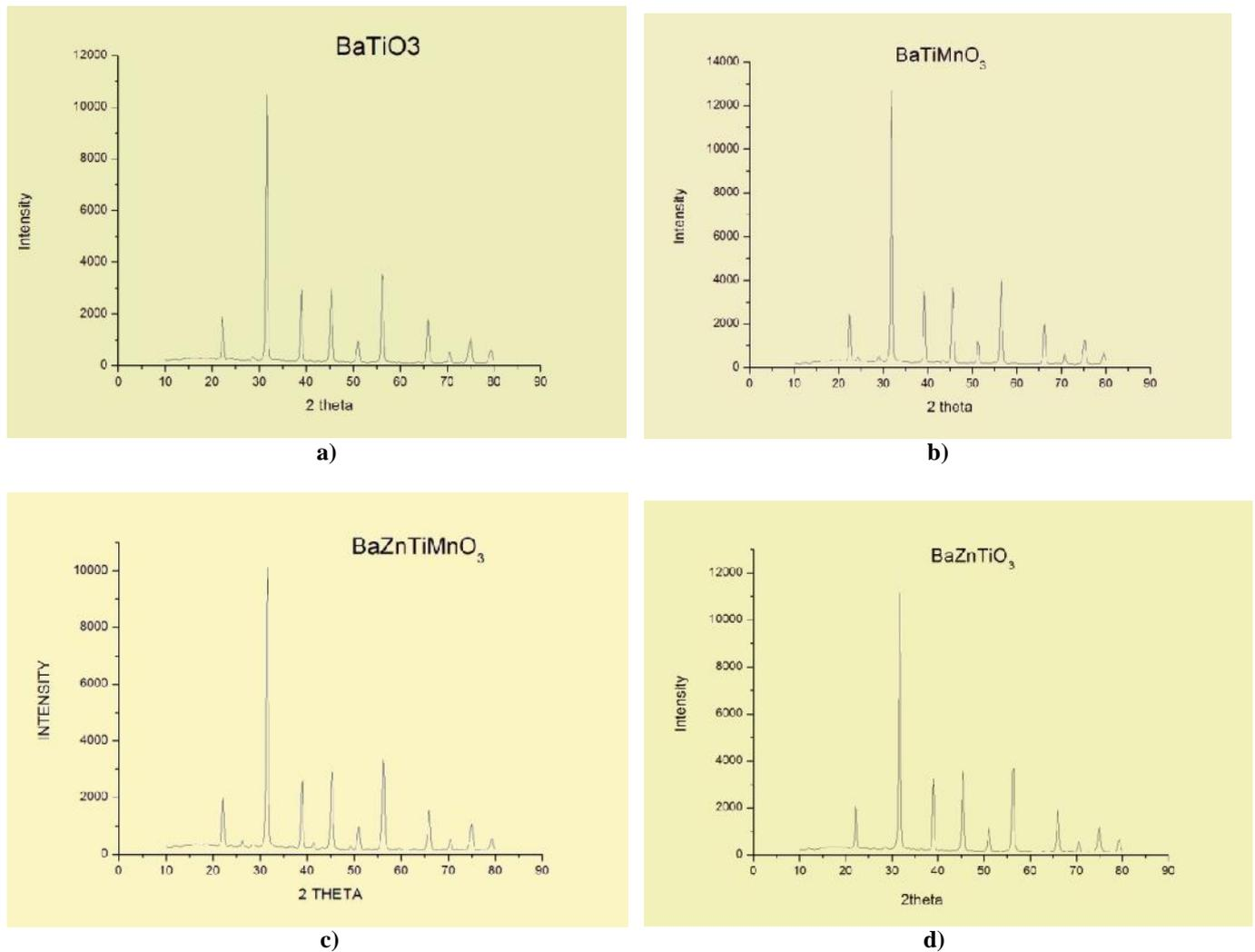
Figure 2(a-d): The x-ray diffraction (XRD) patterns of  $\text{BaTiO}_3$ ,  $\text{Ba}_{0.95}\text{Zn}_{0.05}\text{TiO}_3$ ,  $\text{BaTi}_{0.95}\text{Mn}_{0.05}\text{O}_3$  and  $\text{Ba}_{0.95}\text{Zn}_{0.05}\text{Ti}_{0.95}\text{Mn}_{0.05}\text{O}_3$
