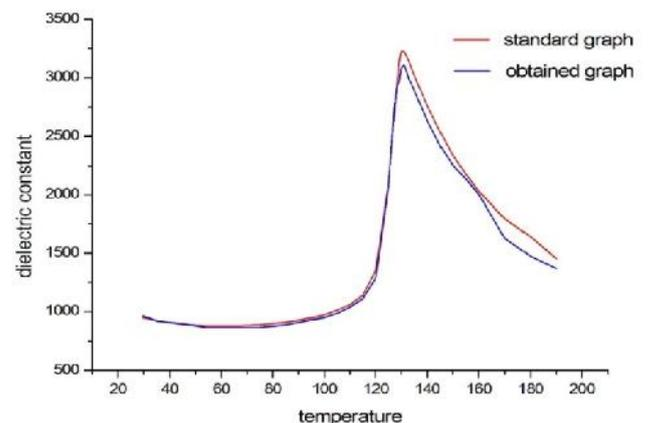
Figure 3. Variation of dielectric constant as a function of temperature of pure  $\text{BaTiO}_3$  sample and is compared with standard value
