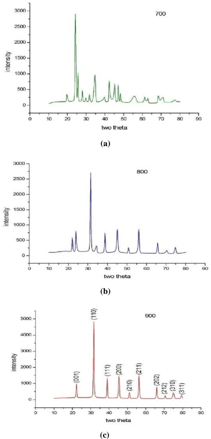
Figure 1 (a-c): X-Ray Diffraction pattern of BaTiO<sub>3</sub> ceramics sintered at various temperatures
