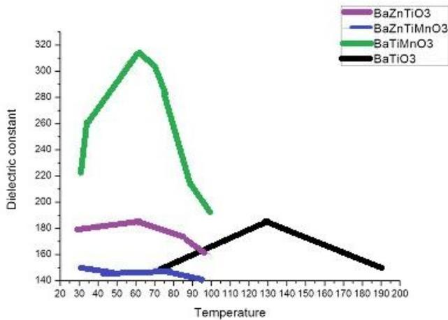
**Figure 4. Dielectric vs temperature graph for BaTiO<sub>3</sub>, Ba<sub>0.95</sub>Zn<sub>0.05</sub>TiO<sub>3</sub>, BaTi<sub>0.95</sub>Mn<sub>0.05</sub>O<sub>3</sub> and Ba<sub>0.95</sub>Zn<sub>0.05</sub>Ti<sub>0.95</sub>Mn<sub>0.05</sub>O<sub>3</sub>**
