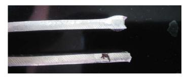
Figure 1. Failed tensile test specimen showing cup and cone type fracture
