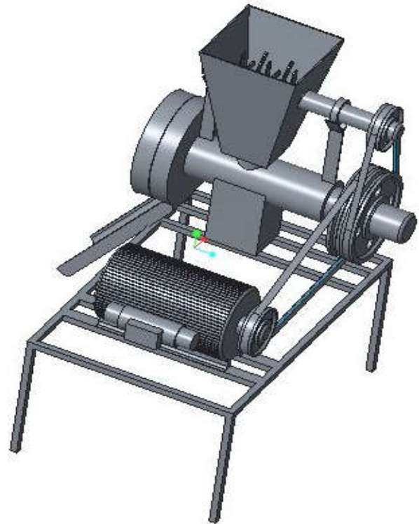
Fig. 3. Working Mechanism of ginger garlic pasting machine
