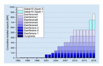
Figure 12. The cumulative installed capacity of wind farms in Egypt from 2001 till the end of 2016 (Noha Saad Hussein *et al.*, 2016)
