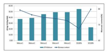
Figure 4. AT<sub>4</sub> values and biomass content according to mixing ratio
