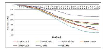
Figure 3. Reduction of pressure by mixing ratio
