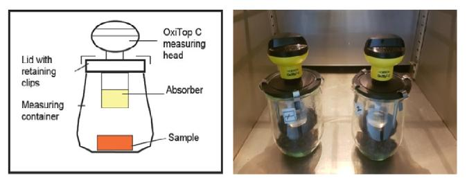
Figure 1. AT<sub>4</sub> schematics (Kim et al., 2009) and measurement device
