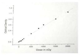
2. Calibration curve of FBX dosimeter for high dose
