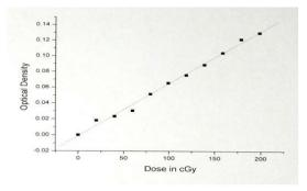
1. Calibration curve of FBX dosimeter for low dose
