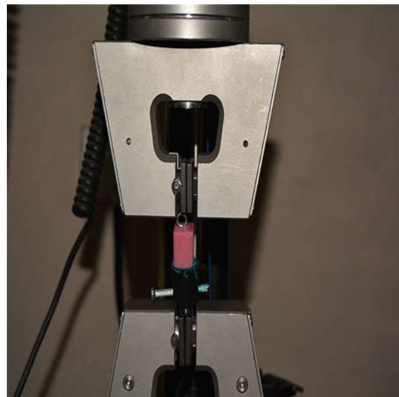
Fig. 8. Each specimen was then attached to the universal testing machine
