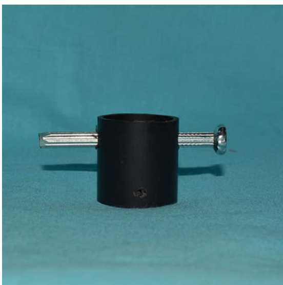
Fig. 3. A metal rod inserted into 2 centered holes to provide retention The specimen surface polished with a 320-grit silicon carbide paper
