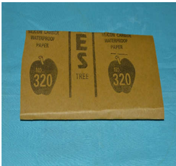
Fig. 2. The specimen surface polished with a 320-grit silicon carbide paper
