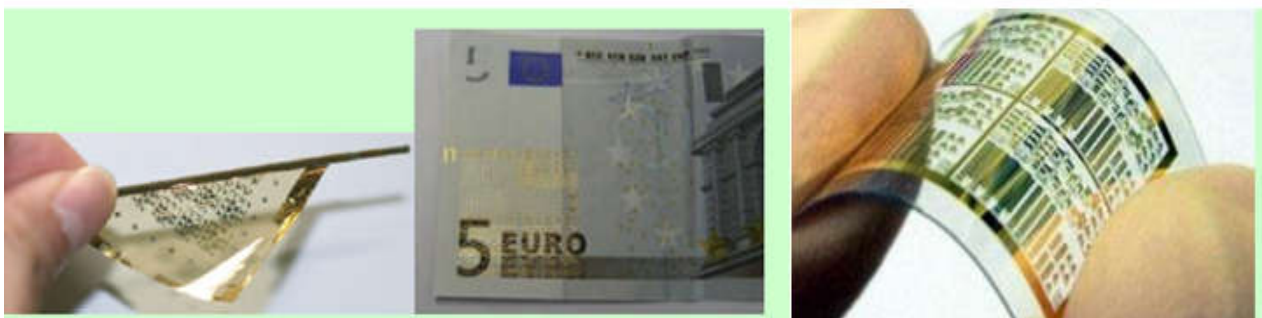
Figure 9. OTFTs make for good anti-counterfeiting features in banknotes. Left: Polymer substrate with functional OTFTs wrapped around a cylinder with a radius of 300 \mu\text{m} .
