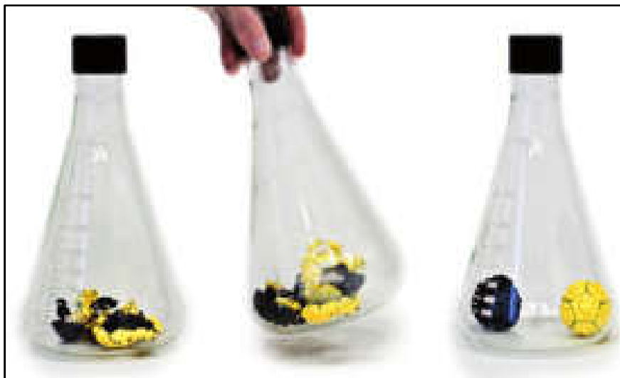
Figure 8. Self-Assembling Materials 6 . Demonstration of self-assembly and molecular chirality, or right-handed and left-handed patterns of attraction. Opposing attraction patterns in the self-assembly units allowed for the parts to sort themselves when combined and shaken randomly. The yellow units and black units eventually self-assemble into two distinct structures, demonstrating error-correction throughout the assembly process. The molecular structures in this exhibit were based on the Polio Virus capsid
