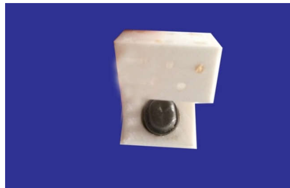
Figure 2. Master metal die seated inside special tray. Special tray fabricated using 3D Printer
