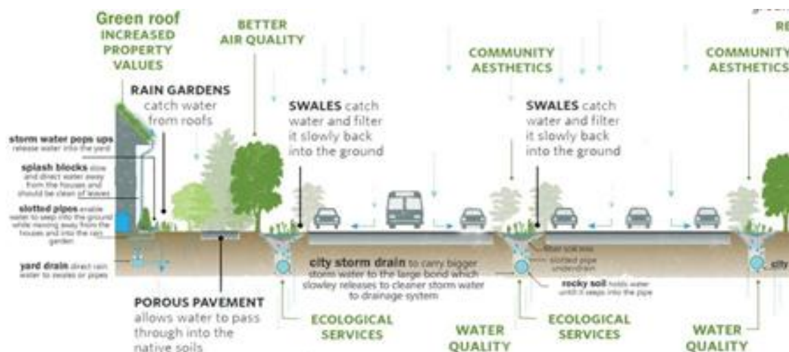
Fig. 9. Section A-A in the proposed design for housing zone and street zone in New-Mansoura city (Author, 2019)
