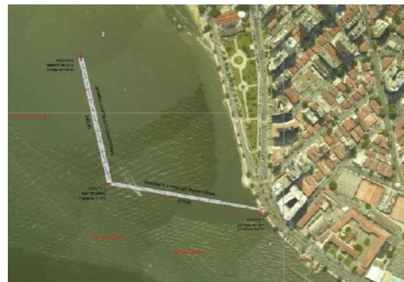
Fig.3. The submerged barrier for the southeast zone in Santos, Brazil (Santos city hall, 2019)
