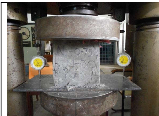
Fig. 1 Details of dial gauge positions and test setup
