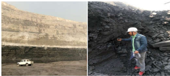
Fig. 2. Vertical profile of coal seam showing the bottom Turra seam and collection of coal samples from the exposed seam section
