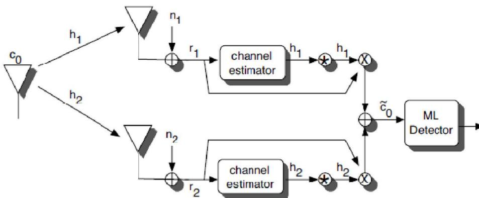
Fig. 3. Maximum Ratio Combining with 1 Tx and 2 Rx antenna (Cho et al., 2010)
