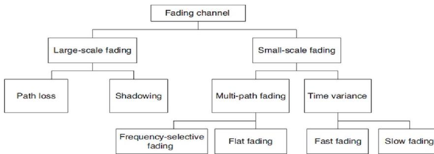
Fig. 1. Classification of fading channels (Cho et al., 2010)
