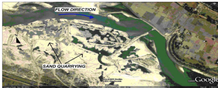
Fig. 9: Image showing the evidence of sand quarrying activity, which is the weakest location of next shifting of Damodar River in high discharge period
