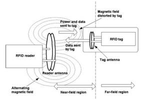
Fig. 2. Showing the schematic of near-field coupling between a reader and a tag [9].
