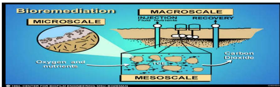
Fig. 13: In-situ bioremediation. Source: Stewart (2008)
