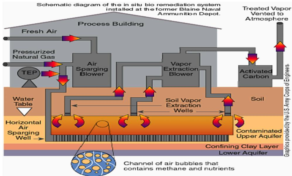
Fig. 11. Air-Sparging. Source: Stewart (2008)
