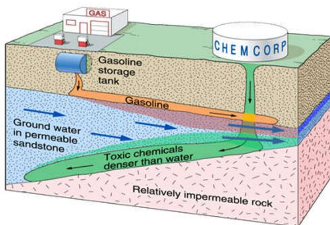
Fig. 4. Underground Storage Tank. Source: Plummer *et al.* (2005)
