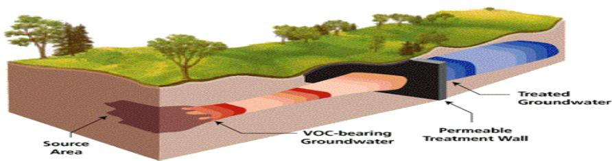
Fig. 12. Permeable Reactive Barriers (PRBS). Source: Reddy (2008)
