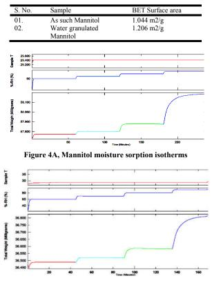
Figure 4B. Water granulated Mannitol moisture sorption isotherms
