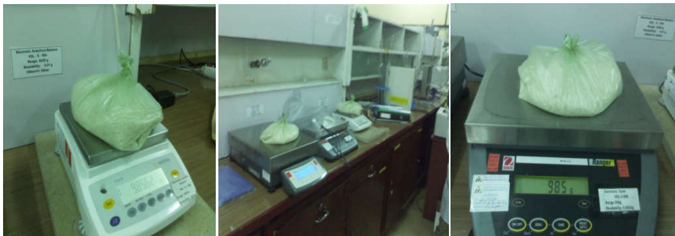
Figure 1. The mass of a 1 kg sample as measured by researchers in mass laboratory of Metrological institute of Ethiopia (NMI) for comparison (traceability)
