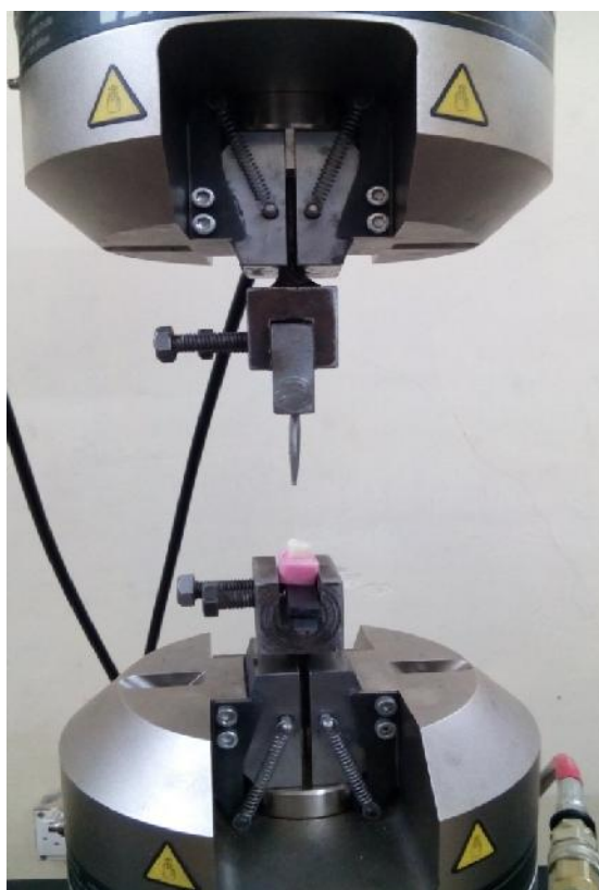
Figure 2. Specially adapted jig for testing of the core material
