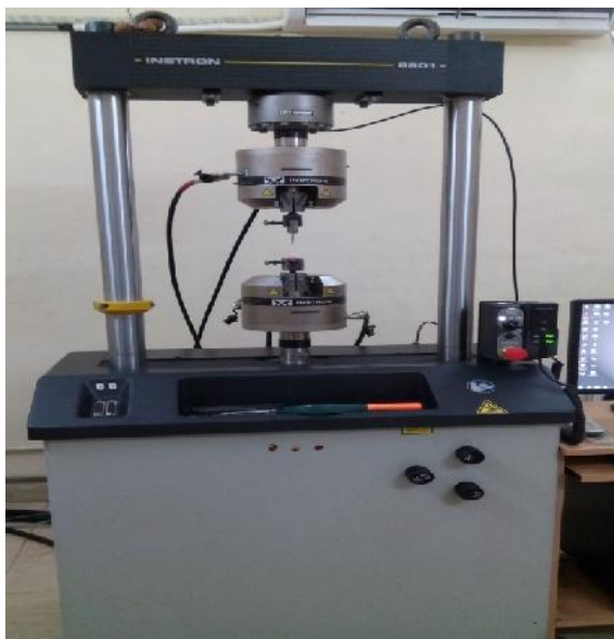
Figure 1. Intron Universal testing machine - 8801 used for testing
