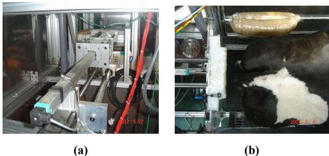
Figure 24. Designed fixed cow bar for manipulator protection (a) LVDT sensor with fixed bar driver (b) Ultrasonic sensor with fixed bar driver
