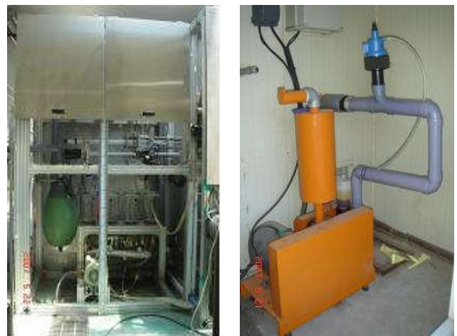
Figure 22. Vacuum generating system
