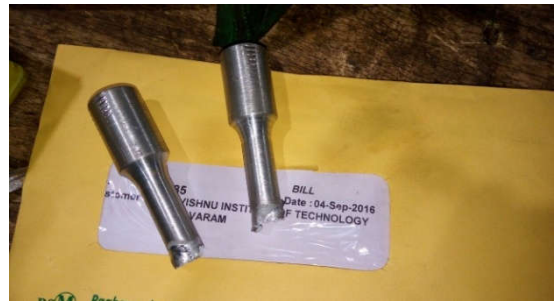
Fig. 15. Cup and Cone shape shown in sample model
