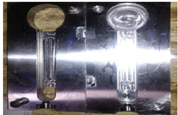
Fig. 10. Core and cavity of connecting rod
