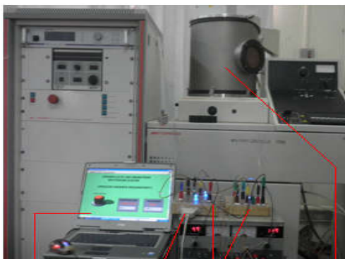
Laptop with parallel port Parallel port interface digital interface board Vacuum deposition system
