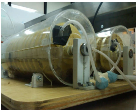
Fig. 4. Reactor tank 1 SSE (left-side) and reactor tank 2 CIB (right-side)
