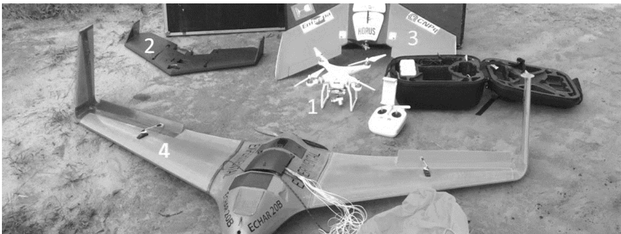
Fig.2. UAVs used in this study: Phantom 3 Professional (1); Swinglet Cam (2), Isis (3); and Echar 20B (4)
