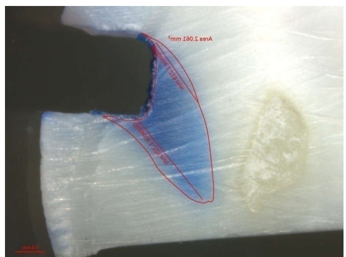
Fig. 3b. Measurement of depth and area of dye penetration by using LEXT software
