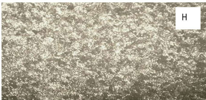
Plate VIII. As received high carbon steel the structure consists of tempered martensite
