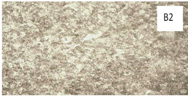
(B2) The structure is pearlite in predominantly martensitic matrix. Samples austenitized at 880°C. 2% Nital etch. Mag. X 100
