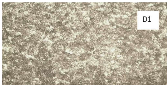
(D1) Microstructure of 1.14% carbon steel quenched Toluene; heated at 840°C the structure consists of martensite in coarse form and retained austenite
