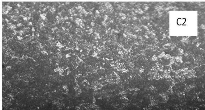
(C2) The structure consists of coarse structure of martensite formed in the matrix of pearlite. Samples austenitized at 880°C. 2% Nital etch. Mag. X 100
