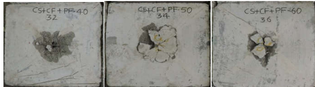
Fig. 10. Crack pattern of M60+CF+PF (40 mm, 50 mm, 60 mm)
