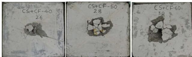
Fig. 9. Crack pattern of M60+CF (40 mm, 50 mm, 60 mm)
