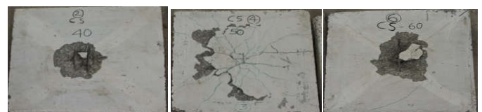
Fig. 8. Crack pattern of CS (40 mm, 50 mm, 60 mm)
