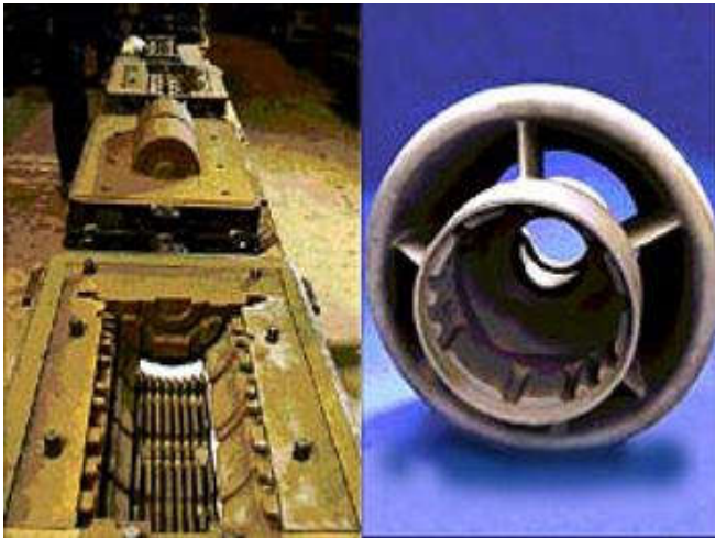
Figure 1. Half mould with cores and an example of a cast air intake for a turbocharger
