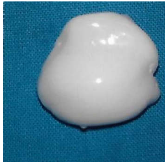
Figure 6. Wax pattern invested and processed with the mixture of clear heat cure acrylic resin and zinc oxide powder
