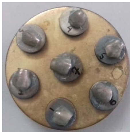
Fig. 4. section teeth sample after gold-palladium sputter coating
