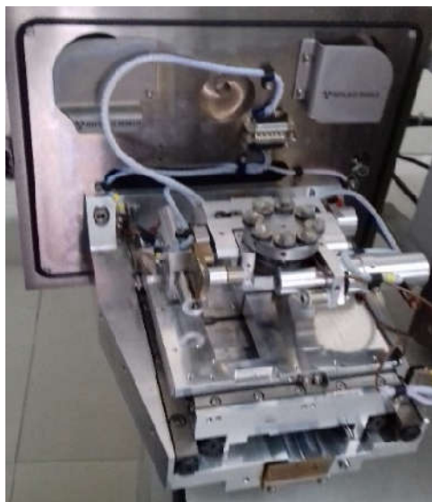
Fig. 6. Teeth sample placed in SEM (LEO 435VF)
