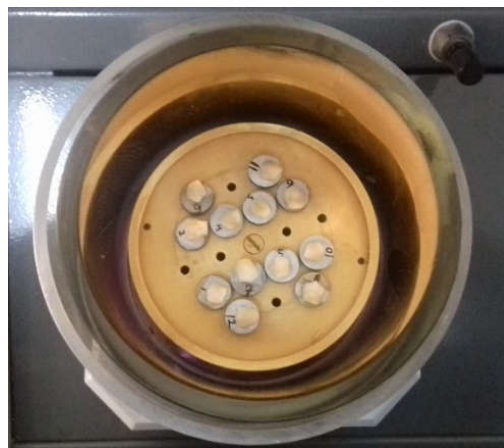
Fig. 3. Sectioned teeth placed in in sputter coater (BAL-TEC SCD 005)
