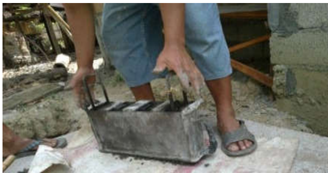
Figure 8. Casting the mixture with the Molder
