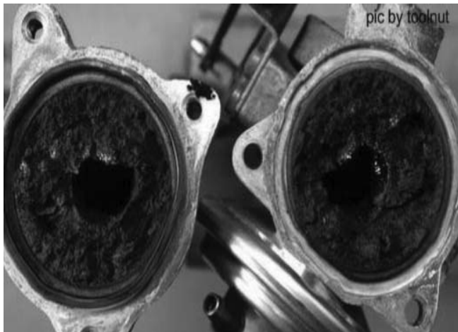
Figure 2. Fouling in EGR cooler (Abd-elhady et al., 2011)
