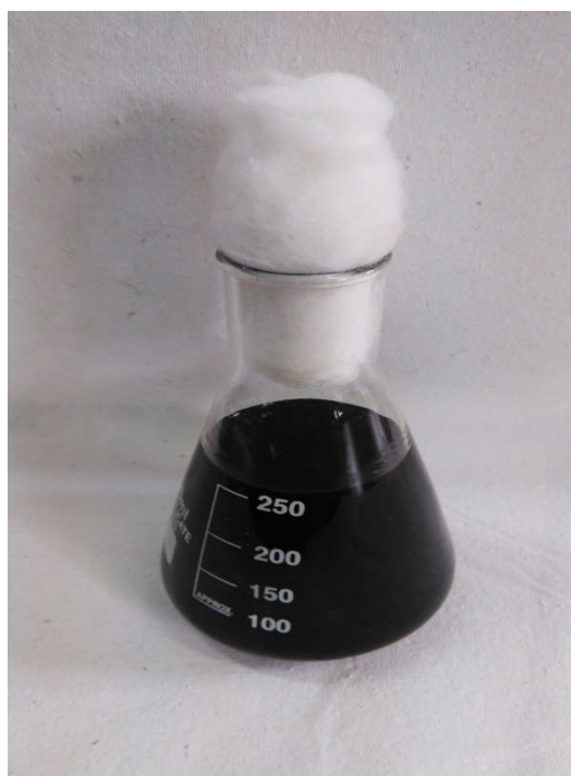
Figure 2. Lignin Extract. It is the source of lignin which could be utilized by microorganisms which are lignin degraders. This is used as carbon source for MSML Medium
