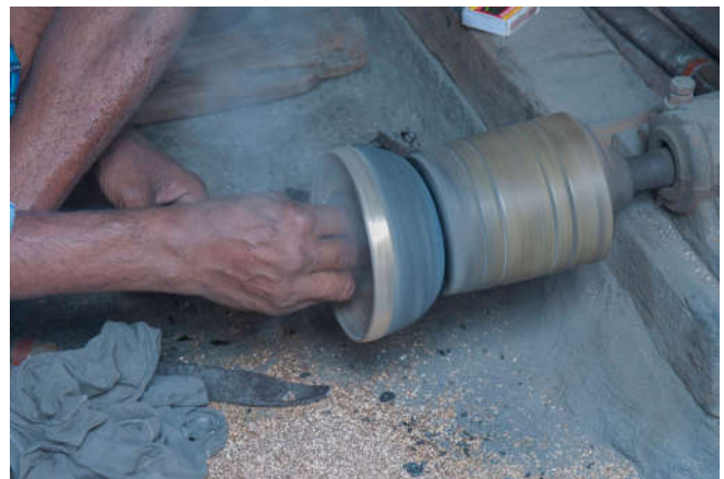
Figure 2. The finishing process of metal bowl in workshop
