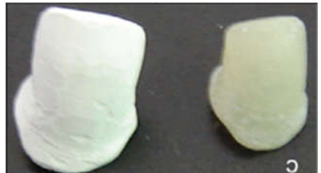
Fig. 2. Coping before and after sintering
