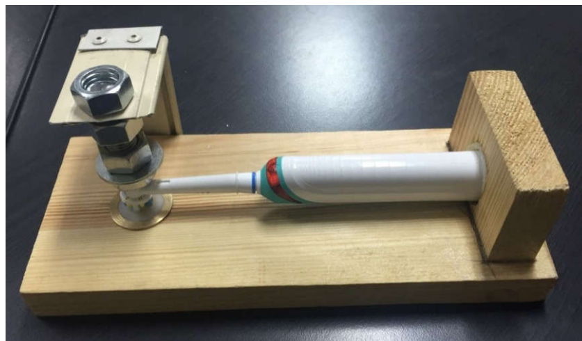
Figure 1. The device used in brushing (wear abrasion test)
