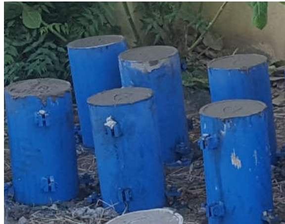
Figure 11. Preservation of test pieces before release
