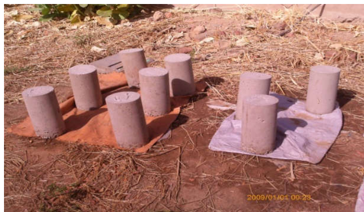
Figure 12. Samples exposed to covered suns with polyane films. Figure 13: Samples exposed to suns covered with jute webs
