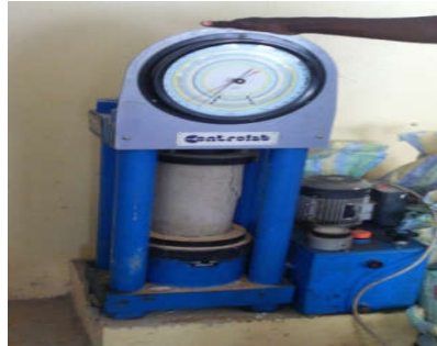
Figure 17: Placement of a test piece in the machine
