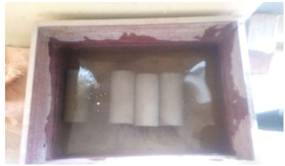
Figure 16: Samples stored in water at 100% RH in an ambient laboratory climate
