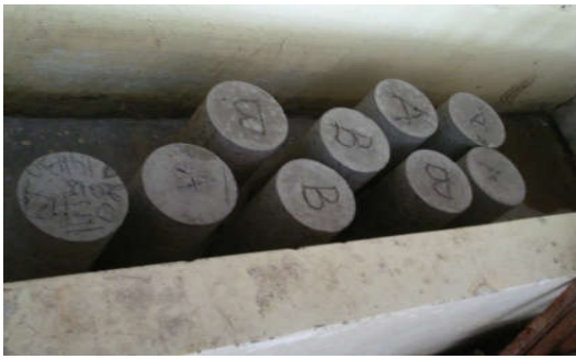
Figure 15: Samples in the shade in the open air (without cover) in an ambient laboratory climate
