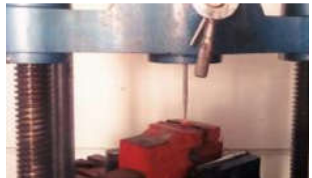
Figure 6. Resin mounting and placement of specimen in Universal testing machine
