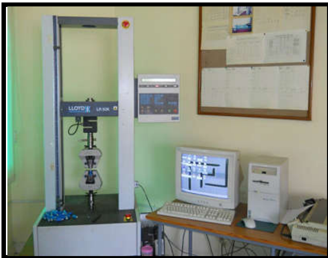
Figure 8. Universal Testing machine (Lloyd instruments) with computer console for recording readings of bond strength testing.
