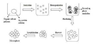
Figure 4. Solvent removal/ Evaporation method Microspheres preparation
