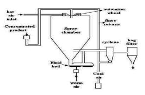
Figure 6. Spray drying method for Microsphere preparation
