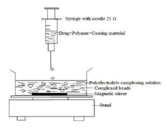
Figure 5. By Ion tropic gelation method for Microspheres preparation
