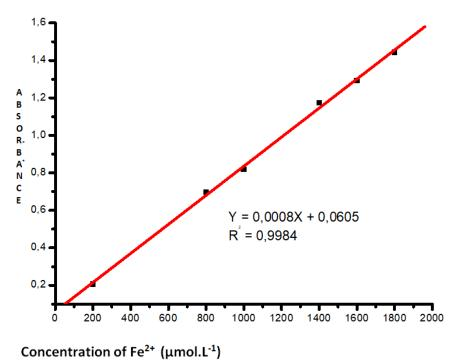
Figure 8. Calibration curve of Fe<sup>2+</sup>
