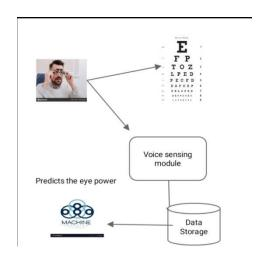
**Voice Module:** The Voice Module has the sensor which used to get the voice from the individual and check with the Snellan chart words or numbers and this matches with it by the arduino programming.
